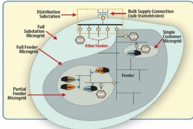
***A microgrid is scalable to serve a single customer or a larger section of the distribution system***
