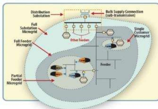
Figure 5: A microgrid is scalable to serve a single customer or a larger section of the distribution system.<sup>16</sup>
