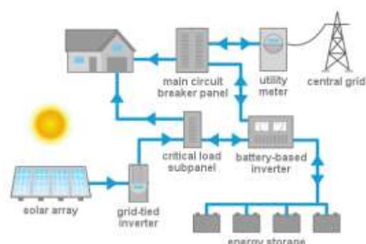
Figure 4: AC-Coupled Solar and Storage System
