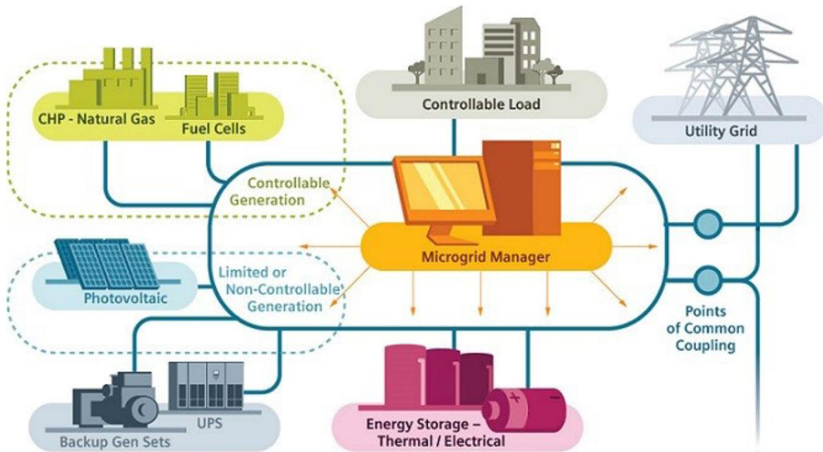
Figure 1. Microgrid with Supervisory controls
