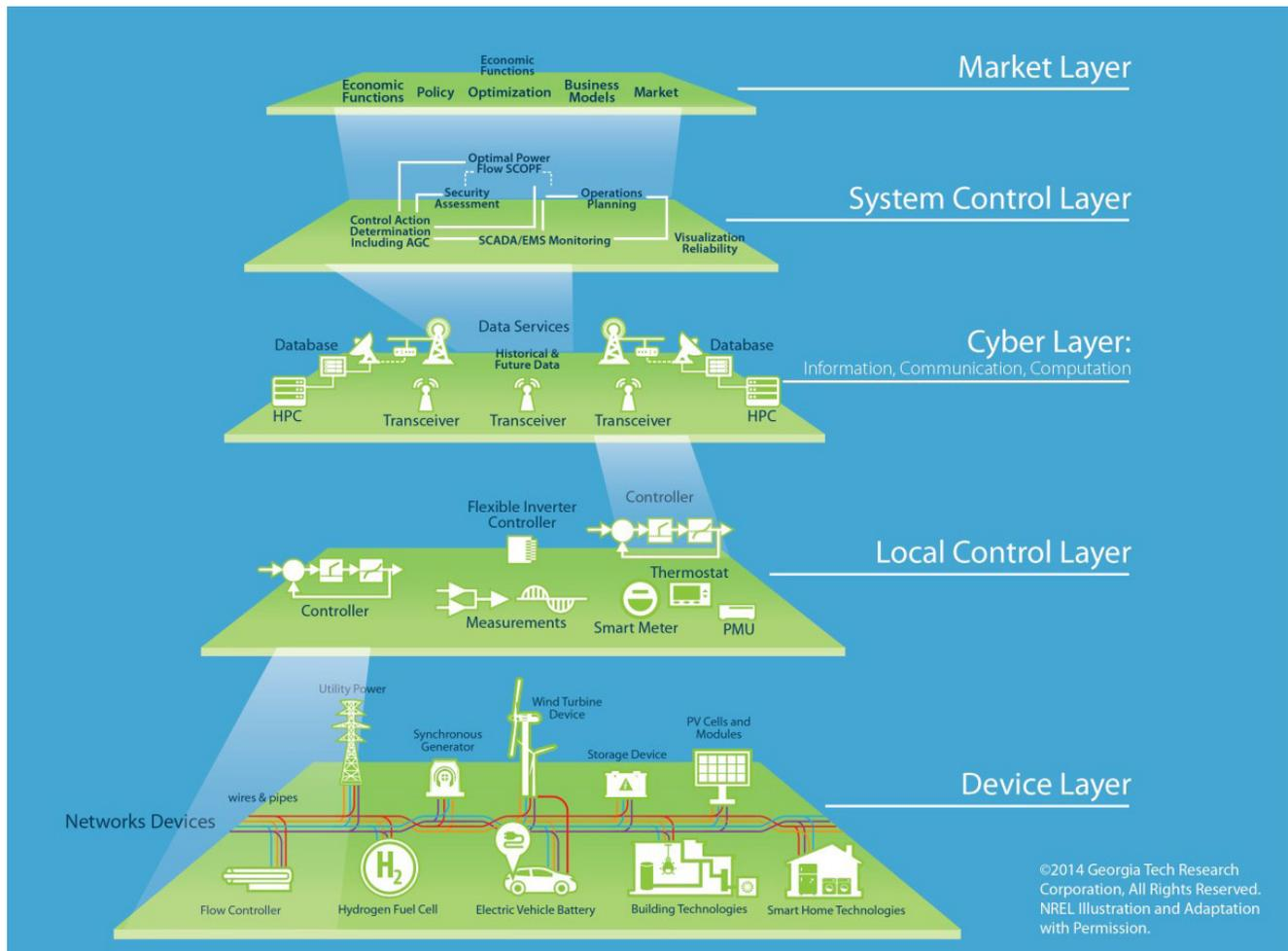
Figure 3. Illustration of the 5 Layers of Communication in a Microgrid
