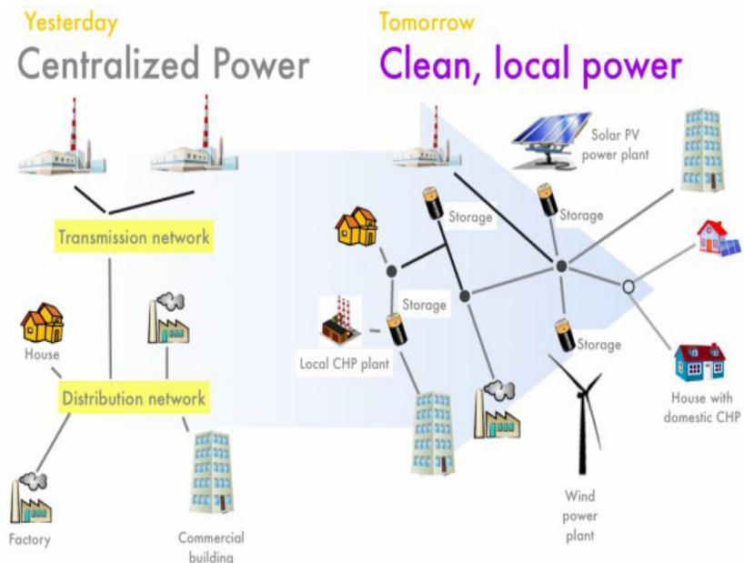
Figure 2. Comparison of Centralized Power system vs Microgrid
